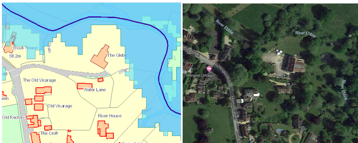
Above left: EA flood zones 2 & 3 indicated in blue block. Above right: Google aerial image showing the new house and garage in situ
